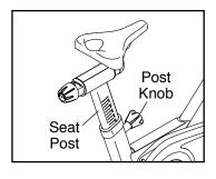
knob. Make sure that the post knob is engaged in an adjustment hole. IMPORTANT: Do not adjust the seat post beyond the stop mark on the seat post.
