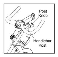
Make sure that the post knob is engaged in an adjustment hole. IMPORTANT: Do not adjust the handlebar post beyond the stop mark on the handlebar post.
