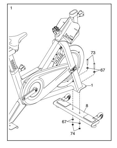
2. Attach the Rear Stabilizer (7) to the Frame (1) with two M10 x 50mm Button Patch Bolts (73), four M10 Washers (67), and two M10 Locknuts (74).
